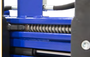
Standard V2A compression spring
