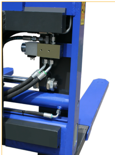
Solenoid valve mounted protected in the frame
