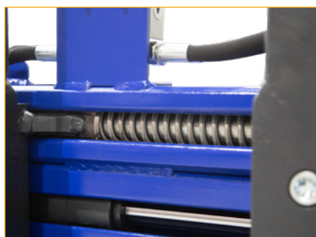
V2A compression spring (no gas pressure cylinders)
